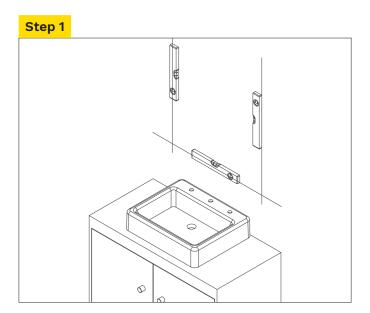
With your level plumb, mark a vertical line on the wall where the edge of the mirror is to be installed.
