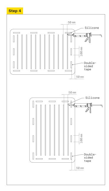
Cut 100 mm strips of double-sided tape and apply 50 mm in from the edge of the mirror as per diagram.
