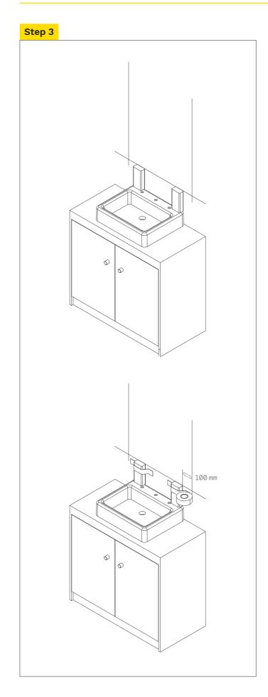
Tape packers to wall approx 100 mm in from each end of the mirror location.
