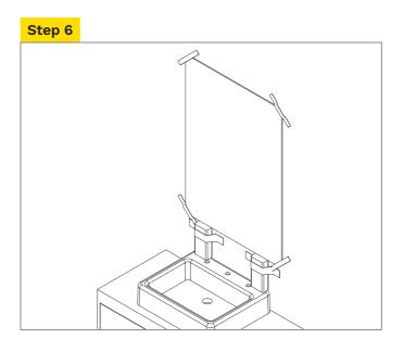
Apply tape to each corner of mirror to ensure mirror does not move.
