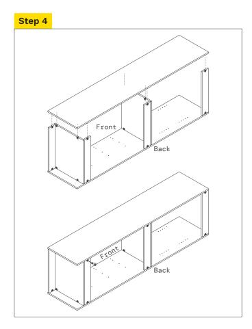
Place side on top over cam bolts and tighten cams.
