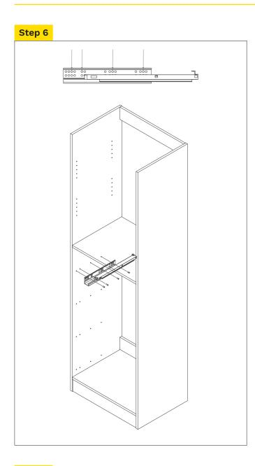
Fix runners L (B) and R (H) to tower sides, screwing euro screw into third hole in top row (Exploded image).
