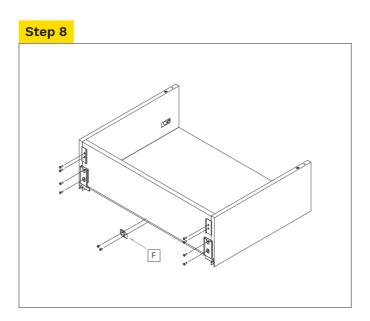
Secure drawer back to bracket using screw.
