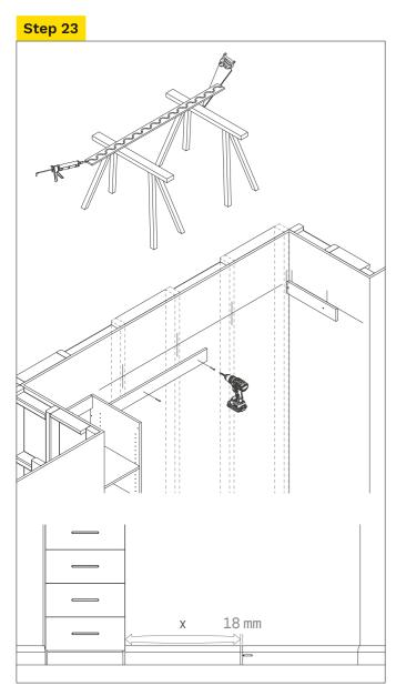
Apply liquid nails to back of cleat in radio wave pattern and screw cleat to wall into stud.
