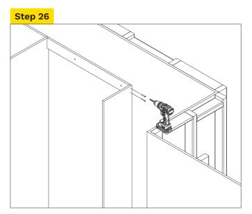
Fix divider to back cleat with a minimum of 2 x 40 mm screws.
