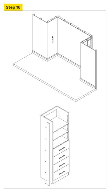
Check wall for plumb, place level on wall.
