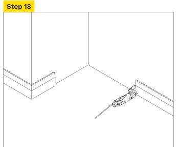
Use multi tool to cut and remove skirting where tower to be installed.
