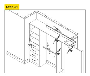
Using caulking, gap all connections between board and wall or board and board.
