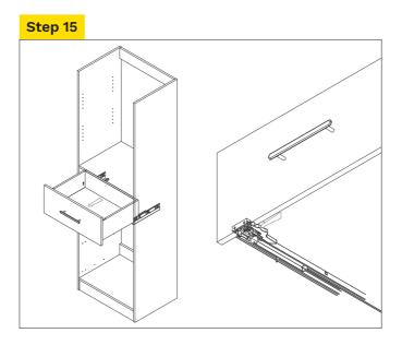
If required, to remove the drawer, extend the drawer, place hands under drawer, locating the brackets on each side and push levers in on drawer. This will release, lifting drawer off runner.
