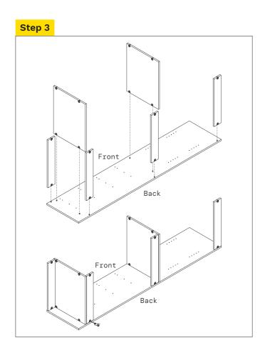
Place nailers over cam bolts and tighten.
