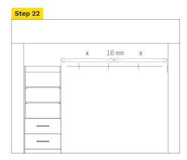
Measure from tower to where the divider is to be located. (max divider span 1200 mm).
