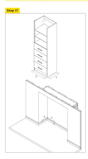
Measure the width and depth of tower and mark skirting with pencil (be sure to include the infill if infill required).
