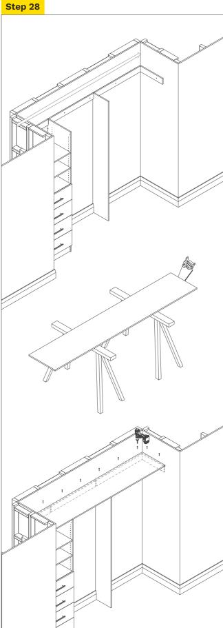
Measure top shelf width ensuring you check the walls are square using a square edge.
