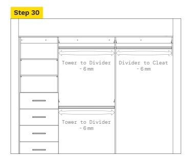
Measure distance between board (tower to divider and (divider to side cleat) and deduct 6 mm off overall width.
