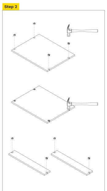
Hammer cams into nailers, toe, deck and fixed shelf.
