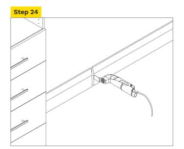
Use a multi tool to cut and remove skirt.
