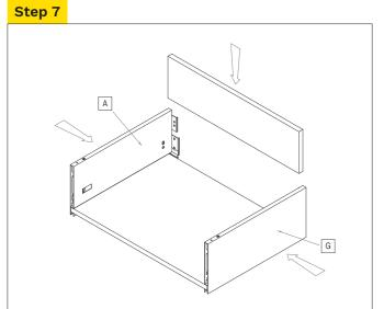
Slide drawer sides A and G into drawer base. Slide drawer back to the inside of the brackets.
